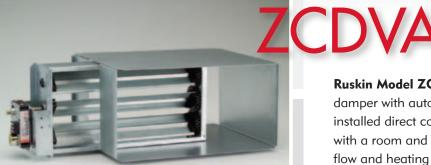
**Ruskin Model ZCDVAV** is a rectangular zone control damper with automatic change over. The factory installed direct coupled modulating actuator, paired with a room and duct thermostat, evenly controls flow and heating to cooling change-over.
